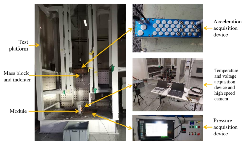
Figure 4. Schematic of the drop-weight test system.
