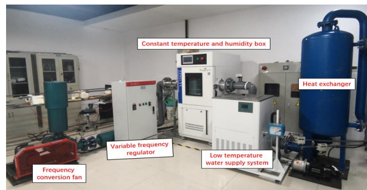
Figure 4. Cooling system experimental platform.
