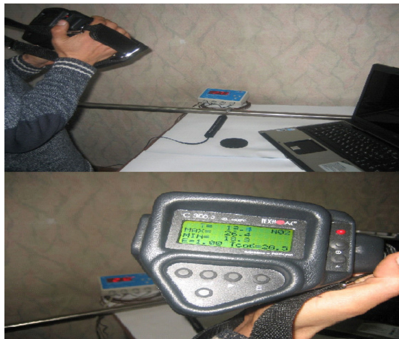
Figure 7. Checking temperature sensors using an infrared pyrometer with 300-3 “Photon”.
