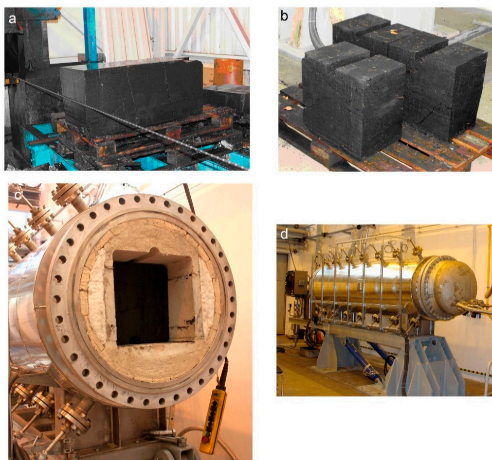
Figure 2. Preparation of coal for gasification. (a) Cutting block of coal, (b) coal blocks with a cut-out fire channel ready to be placed inside the reactor, (c) reaction chamber while loading with coal blocks, (d) reactor prepared for gasification.
