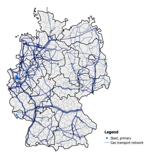
**Figure 4.** Steel production sites in combination with the current gas transportation network. The multiple blue lines show the redundant structure of the German gas transportation network; hence, more than one pipeline supplies the different regions. Based on [26,34] and updated from [27].
