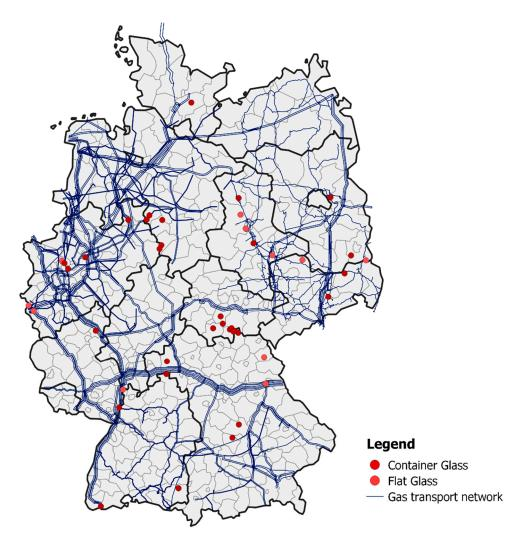
**Figure 6.** Glass production sites in combination with the current gas transportation network. Dark red circles are production sites for container glass and light red circles are production sites for flat glass. Based on [26,34] and updated from [27].
