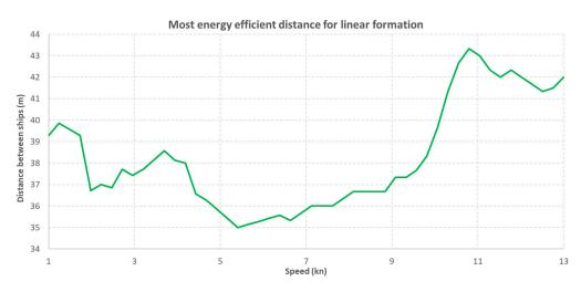
Figure 18. Distance providing the least resistance for a given formation speed in a linear formation.
