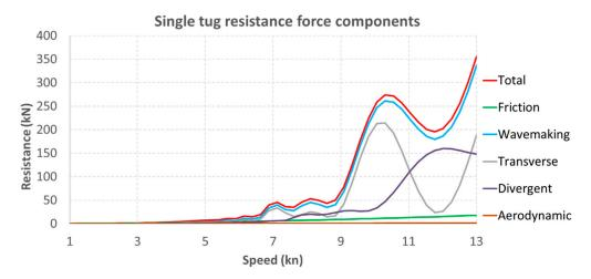
Figure 5. Resistance force components acting on a single tug used in a formation.
