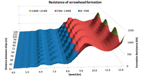
**Figure 13.** Total resistance of a formation composed of four tugboats sailing in a diamond-shaped formation.
