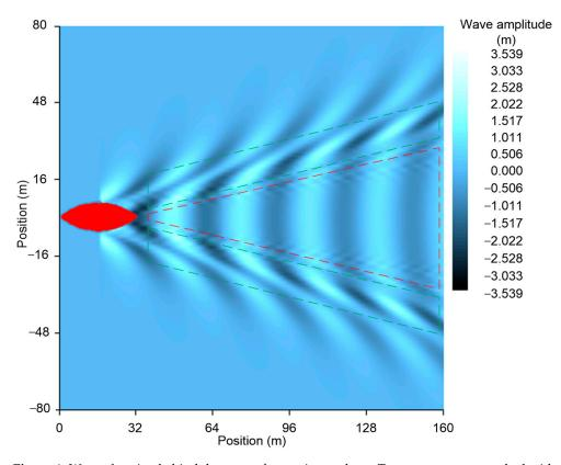
**Figure 4.** Waves forming behind the stern of a moving tugboat. Transverse waves marked with a red outline, divergent waves marked with a green outline.
