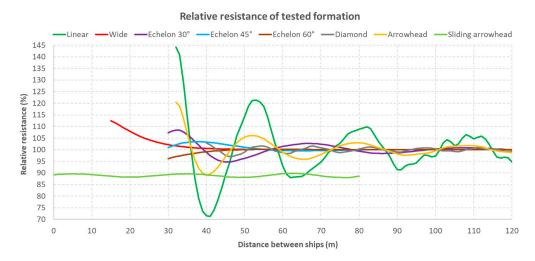
**Figure 15.** Relative value of total drag as a function of ship distance for a given formation in the entire speed range.
