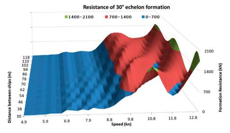
**Figure 9.** Total resistance of a formation consisting of four tugboats sailing in an echelon formation with an angle of  $30^{\circ}$ .
