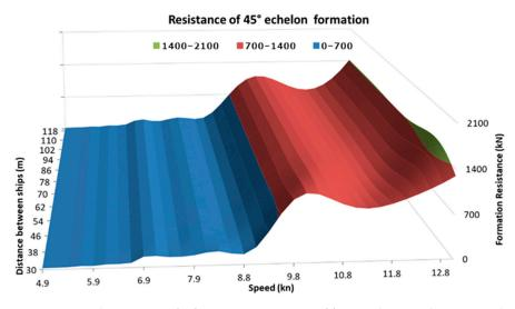
**Figure 10.** Total resistance of a formation consisting of four tugboats sailing in an echelon formation with an angle of  $45^{\circ}$ .
