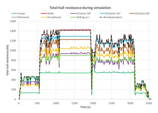
Figure 23. Resistance to motion of four ships moving in formations of various shapes.
