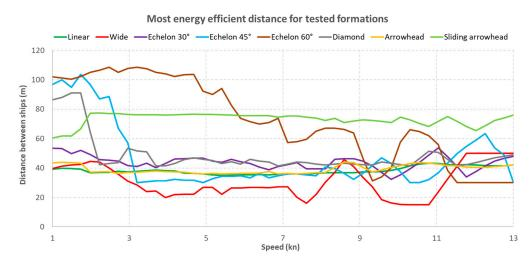
Figure 17. The distance that gives the least resistance for a given speed and shape of the formation.
