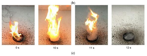
**Figure 4.** Images of flammable liquid fire suppression ( $V_0 \approx 3 \text{ mL}$ ) by carbon dioxide hydrate powder,  $m_g \approx 4 \text{ g}$ : (a) kerosene; (b) motor oil; (c) crude oil ( $d_f \approx 65 \text{ mm}$ ,  $S_f \approx 33 \text{ cm}^2$ ).
