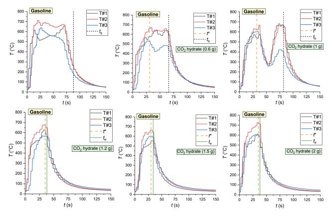
**Figure 12.** Flame temperature variation dynamics (gasoline,  $V_0 \approx 3 \text{ mL}$ ,  $d_f \approx 50 \text{ mm}$ ,  $S_f \approx 20 \text{ cm}^2$ ) without extinguishing and when using CO<sub>2</sub> hydrate powder ( $m_g = 0.6-2 \text{ g}$ ).
