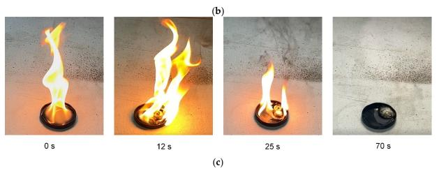
**Figure 2.** Images of gasoline fire suppression ( $V_0 \approx 3 \text{ mL}$ ) with the help of carbon dioxide hydrate in the forms of (a) powder,  $m_{\rm g} \approx 4$  g; (b) tablets,  $m_{\rm g} \approx 1.07$  g; (c) spheres,  $m_{\rm g} \approx 1.42$  g ( $d_{\rm f} \approx 65$  mm,  $S_{\rm f} \approx 33 \ {\rm cm}^2$ ).
