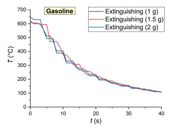
**Figure 14.** Combined experimental trends of the successful suppression of a laboratory-scale gasoline fire ( $V_0 \approx 3 \text{ mL}$ ,  $d_f \approx 50 \text{ mm}$ ,  $S_f \approx 20 \text{ cm}^2$ ) illustrating the flame temperature variation dynamics immediately after the discharge of the extinguishing agent—CO<sub>2</sub> hydrate powder—onto the fire.
