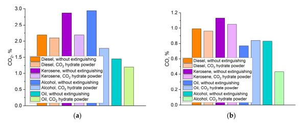
**Figure 10.** Concentrations of CO<sub>2</sub> (**a**) and CO (**b**) from the suppression of flammable liquids (diesel fuel, kerosene, oil, and alcohol) by CO<sub>2</sub> hydrate.
