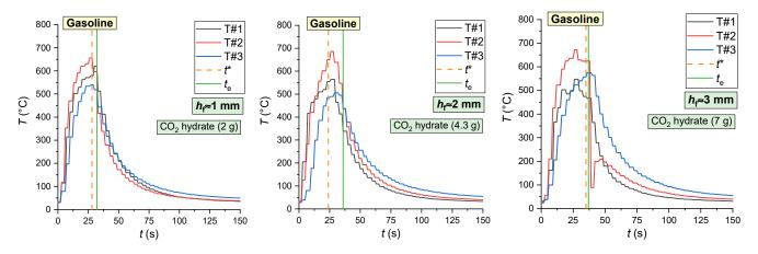
**Figure 15.** Flame temperature variation dynamics (gasoline,  $V_0 \approx 9$  mL,  $d_f \approx 65$  mm,  $S_f \approx 33$  cm<sup>2</sup>) of laboratory-scale fires suppressed by CO<sub>2</sub> hydrate powder with varying thickness of the fuel film (layer).
