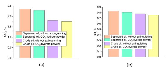
**Figure 11.** Concentrations of  $CO_2$  (**a**) and CO (**b**) released during the suppression of crude and separated oil fire by  $CO_2$  hydrate.
