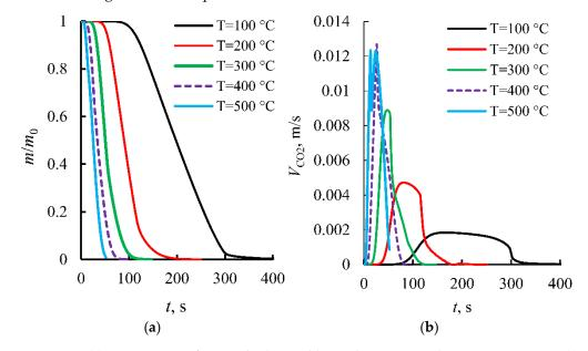
**Figure 18.** (a) Dissociation of a CO<sub>2</sub> hydrate tablet with varying ambient temperature T ( $m_0$  is the initial mass of gas hydrate, the tablet diameter is 20 mm, and the tablet height is 5–6 mm). (b) Carbon dioxide release rate during the dissociation with varying tablet porosity P and ambient gas temperature T.
