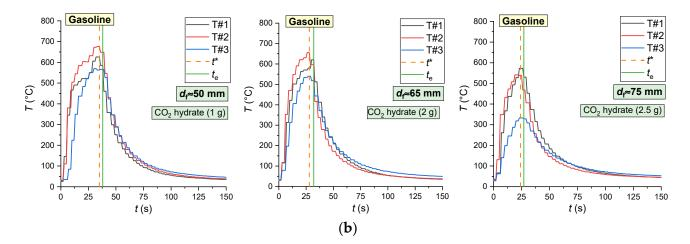
**Figure 13.** Flame temperature variation dynamics for laboratory-scale pool fires of different diameters ( $d_f = 50-75 \text{ mm}$ ) consisting of gasoline ( $V_0 \approx 3 \text{ mL}$ ) and burning without extinguishing (**a**) and when exposed to CO<sub>2</sub> hydrate powder (**b**).
