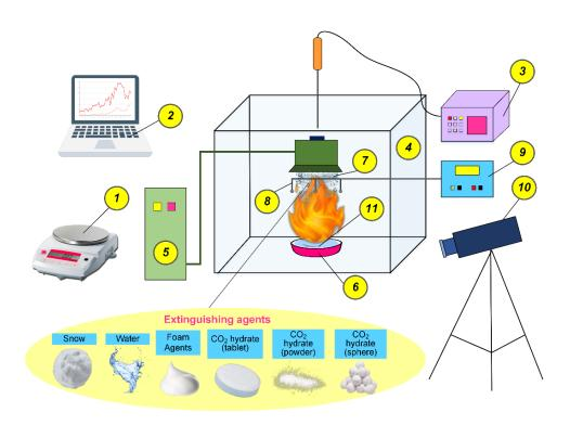
**Figure 1.** Scheme of setup: 1—electronic balance; 2—laptop; 3—gas analyzer; 4—transparent cube; 5—extinguishing agent feeder; 6—container with a burning liquid; 7—extinguishing agent; 8—thermocouple; 9—temperature transmitter; 10—camera; 11—flammable liquid.
