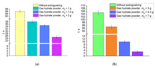
**Figure 5.** Extinction times of gasoline with varying initial volume ( $V_0$ ) burning when no extinguishing agents were used and when in contact with CO<sub>2</sub> hydrate powder with varying initial mass  $m_g$ : (a)  $V_0 \approx 3$  mL; (b)  $V_0 \approx 6$  mL.
