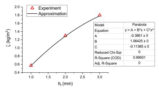
**Figure 16.** CO<sub>2</sub> hydrate powder discharge density per unit area of the flammable liquid versus the thickness of the liquid layer necessary and sufficient for the suppression of a laboratory-scale class B fire.
