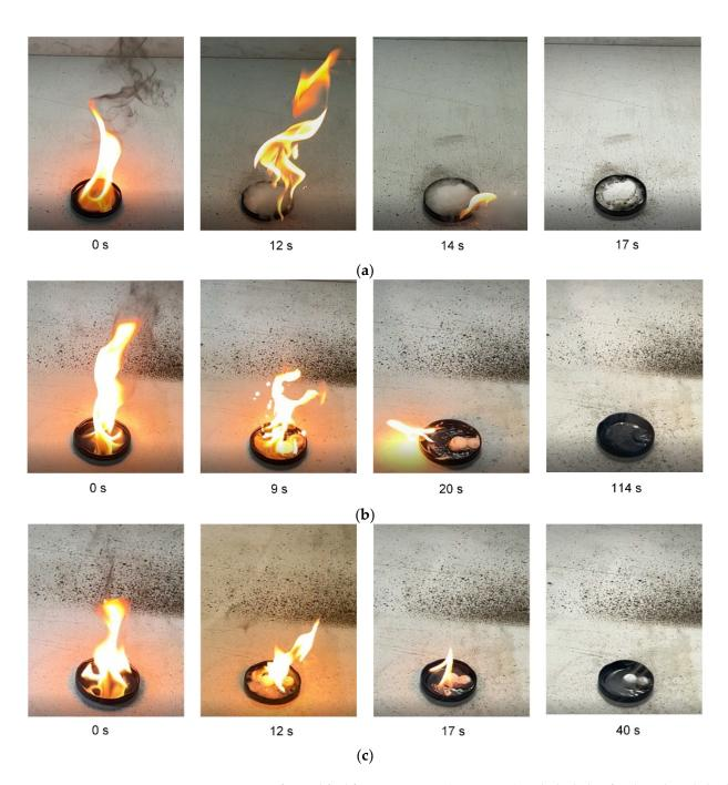
**Figure 3.** Images of Diesel fuel fire suppression ( $V_0 \approx 3 \text{ mL}$ ) with the help of carbon dioxide hydrate in the forms of (**a**)) powder,  $m_g \approx 4$  g; (**b**)) tablets,  $m_g \approx 1.07$  g; (**c**)) spheres,  $m_g \approx 1.42$  g ( $d_f \approx 65$  mm,  $S_f \approx 33$  cm<sup>2</sup>).
