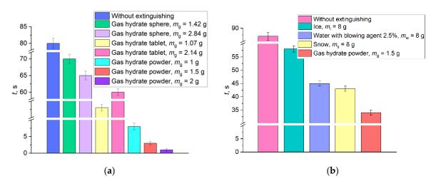
**Figure 8.** Extinction times of a gasoline pool fire ( $V_0 \approx 3$  mL) without extinguishing and when suppressed by (a) CO<sub>2</sub> hydrate in the form of powder, tablets, and spheres with varying initial mass  $m_{g}$ , and (b) ice and water with 2.5% of foaming agent, snow, and CO<sub>2</sub> hydrate powder.
