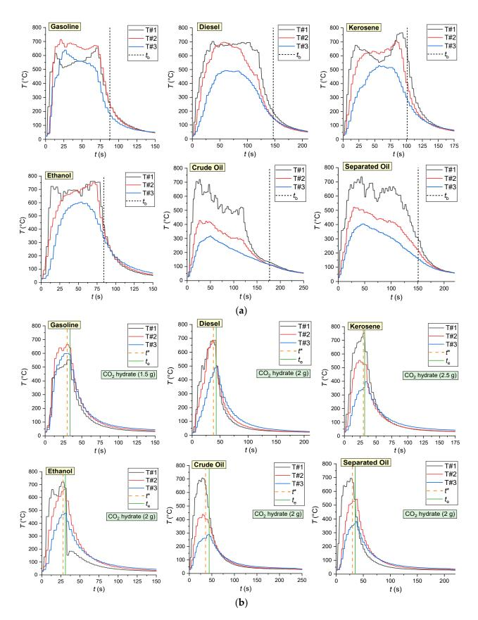
**Figure 17.** Flame temperature variation dynamics of laboratory-scale fires involving different flammable liquids ( $V_0 \approx 3 \text{ mL}$ ,  $d_f \approx 50 \text{ mm}$ ,  $S_f \approx 20 \text{ cm}^2$ ) without extinguishing (**a**) and when suppressed by CO<sub>2</sub> hydrate powder (**b**).
