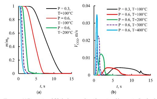
**Figure 19.** (a) Dissociation of CO<sub>2</sub> hydrate powder with varying tablet porosity *P* and ambient gas temperature *T* ( $m_0$  is the initial mass of gas hydrate; the spherical granule diameter is 3 mm). (b) Carbon dioxide release rate during the dissociation with varying *P* and *T*.
