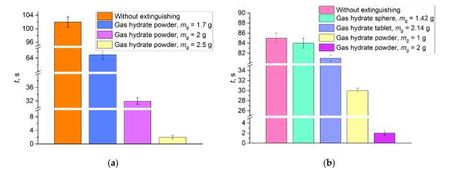
**Figure 7.** Extinction times of (**a**) kerosene ( $V_0 \approx 3 \text{ mL}$ ) and (**b**) alcohol ( $V_0 \approx 3 \text{ mL}$ ) pool fires without extinguishing and when suppressed by CO<sub>2</sub> hydrate in the form of powder, tablets, and spheres with varying initial mass  $m_g$ .
