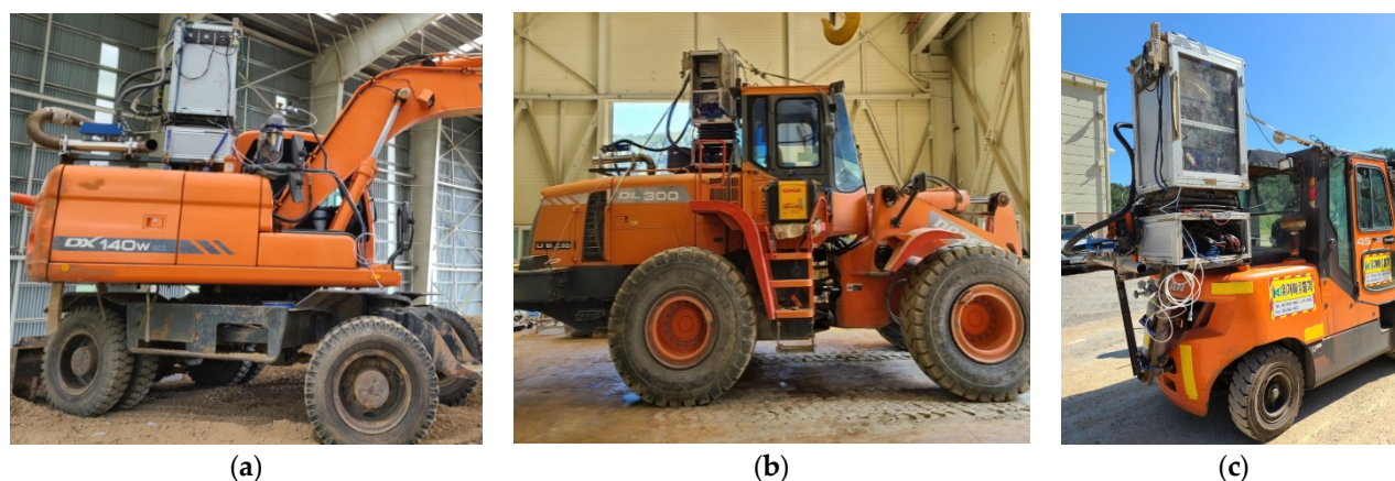
Figure 1. Real-operation of construction machinery with PEMS; (a) Excavator, (b) Wheel loader, (c) Fork-lift.
