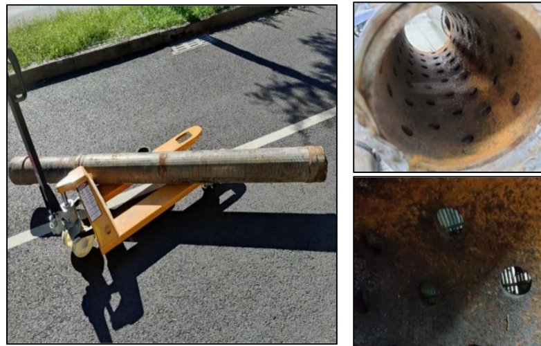
Figure 3. Experiment screen tube and internal conditions.
