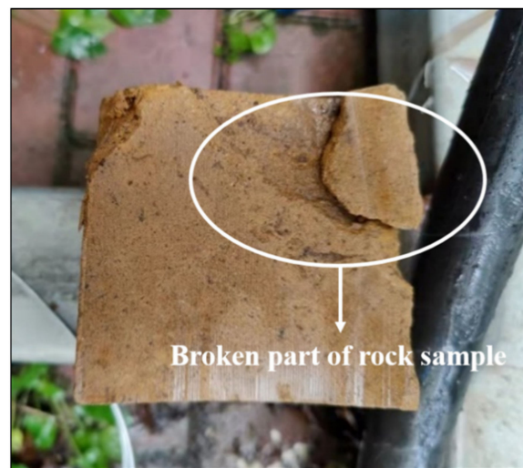
Figure 8. Post-experimental yellow sandstone rock sample.
