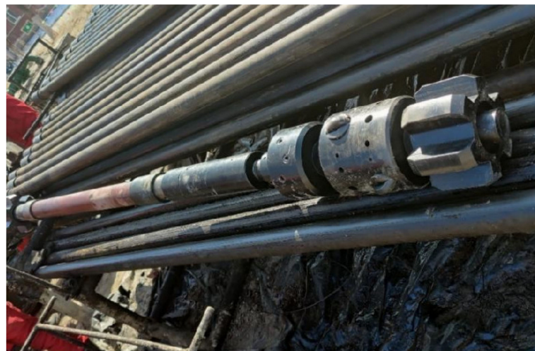
Figure 21. Installation diagram of rotary jet unblock tool.
