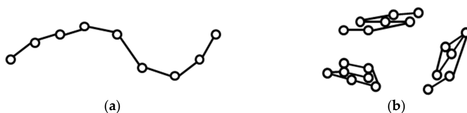
Figure 3. Acrylic polymer macromolecules in a neutral medium (closer to pH = 5–6)—(a); in an acidic medium—(b) (pH < 1).
