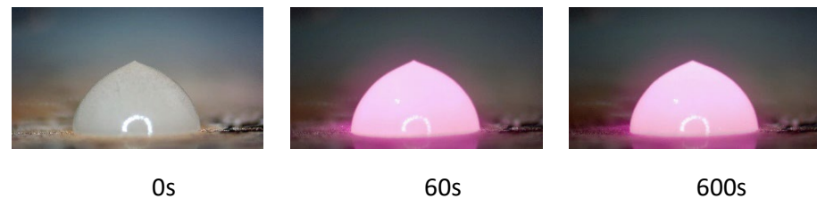
Figure 8. Droplet morphology on the surface of the purple copper plate under the illumination intensity of 3 \text{ W/cm}^2 .
