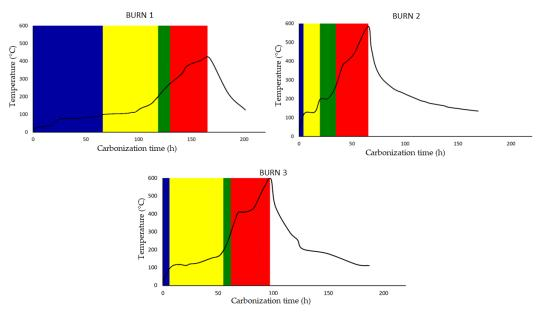
**Figure 7.** Heating ramps during carbonization in three burnings of modified Brazilian beehive kilns. Blue color = phase 1, yellow color = phase 2, green color = phase 3, red color = phase 4, white color = phase 5. This carbonization process includes the following species: Guamúchil and Tamarindo.
