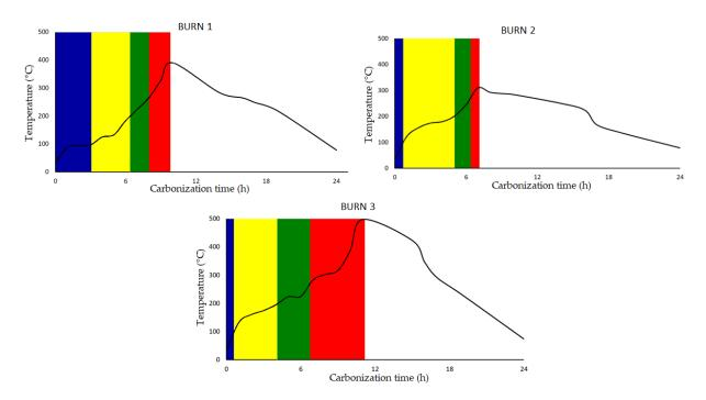
**Figure 9.** Heating ramps during carbonization in three burnings of industrial metal kilns. Blue color = phase 1, yellow color = phase 2, green color = phase 3, red color = phase 4, white color = phase 5. This carbonization process includes the following species: Ramón, Yaxnic, Zapote, and Zapotillo.
