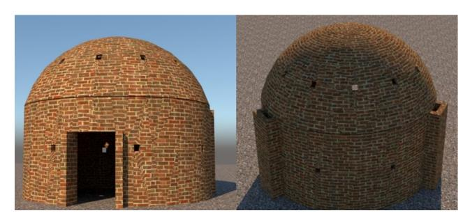
Figure 2. Design of a Brazilian beehive type kiln.
