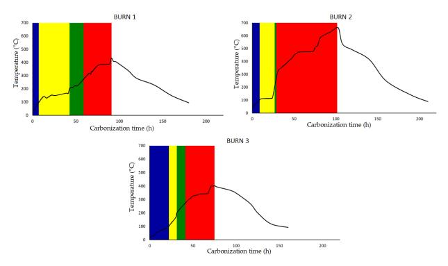
**Figure 8.** Heating ramps during carbonization in three burnings of Argentine half-orange kilns. Blue color = phase 1, yellow color = phase 2, green color = phase 3, red color = phase 4, white color = phase 5. This carbonization process includes the following species: White oak and Red oak.
