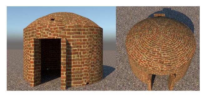
Figure 3. Design of a modified Brazilian beehive type kiln.
