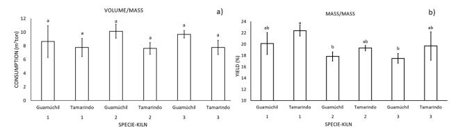
**Figure 10.** (a) Firewood consumption, and (b) charcoal production yield in modified Brazilian behive kilns. Values with the same letter are statistically equal, according to Tukey test ( $p \ge 0.05$ ).
