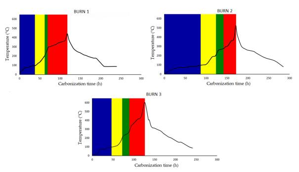
**Figure 6.** Heating ramps during carbonization in three burnings of Brazilian beehive kilns. Blue color = phase 1, yellow color = phase 2, green color = phase 3, red color = phase 4, white color = phase 5. This carbonization process includes the following species: Madrone, White oak, and Red oak.
