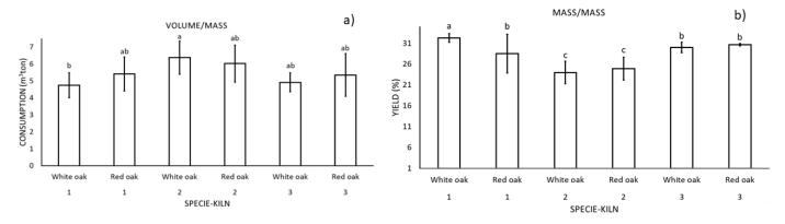
**Figure 11.** (a) Firewood consumption and (b) charcoal production yield in Argentine half-orange kilns. Values with the same letter are statistically equal, according to Tukey test (p > 0.05).
