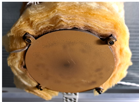
Figure 2. External view of the catalytic reactor.
