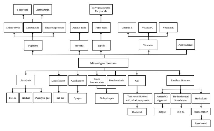
**Figure 1.** Primary processes used for converting microalgal biomass into biofuels, together with the major value-added products harvestable from microalgae.
