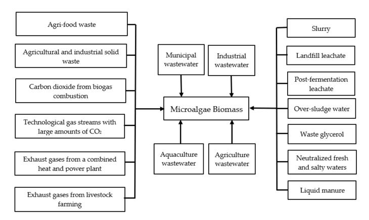
Figure 2. Primary types of waste used for microalgal biomass production.
