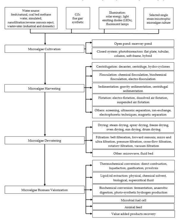
**Figure 4.** The many available process steps in microalgal biomass cultivation and microalgae-tobiofuel conversion.
