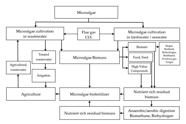
Figure 8. Microalgae biomass in a comprehensive biorefinery concept.
