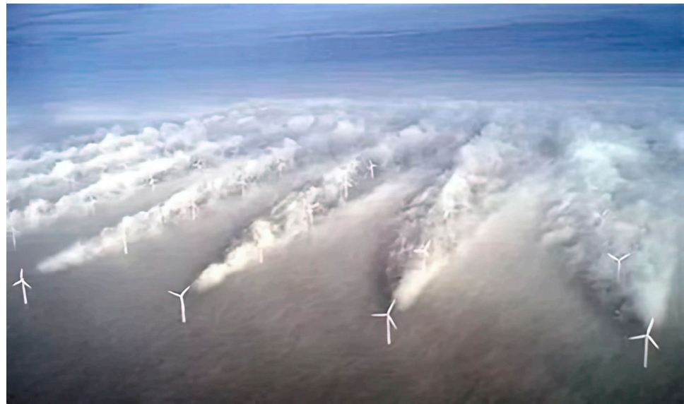
Figure 10. Picture of the wake effect at the Horns Rev offshore wind farm in Denmark [90].
