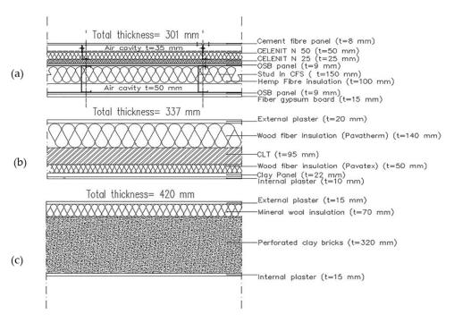
Figure 8. Wall configurations: (a) CFS; (b) CLT; (c) traditional.
