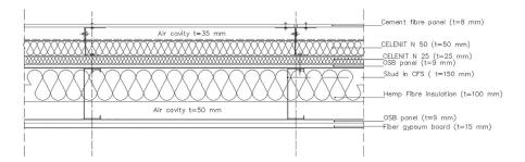
**Figure 3.** External wall section of the British Foundation school.
