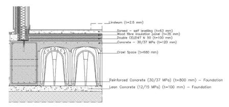
Figure 2. Foundation and ground floor sections.
