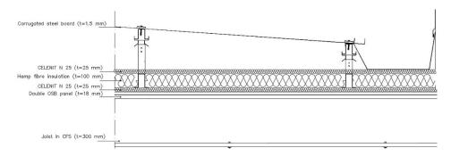
Figure 5. Roof section.
