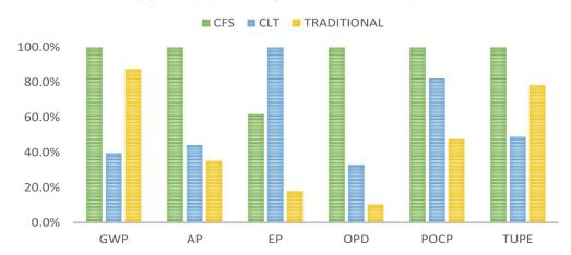
Figure 15. Results of Life Cycle impact assessment: External Wall.
