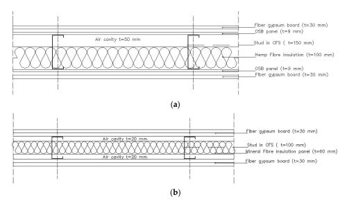
Figure 4. Internal wall sections: (a) load-bearing wall; (b) non-load-bearing wall.
