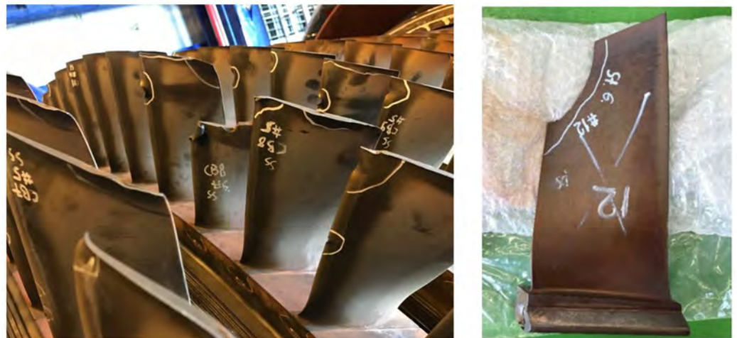
Figure 1. Housing damage on the compressor blades in a gas turbine power plant [1]. Copyright 2019 MDPI.
