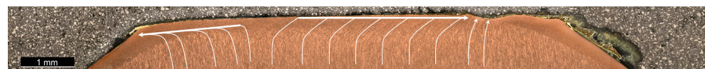
Figure 14. Mushrooming due to radial material flow indicated by white arrows of upper electrode of MC01–TS01 after 1200 spot welds in cross-section.
