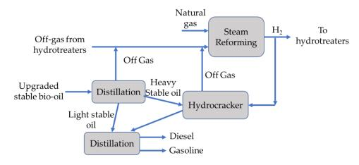
**Figure 4.** Block diagram for hydrocracking and product separation [74].
