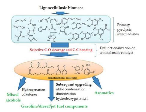
Figure 2. Biofuel production through bio-oil enhancement [50].
