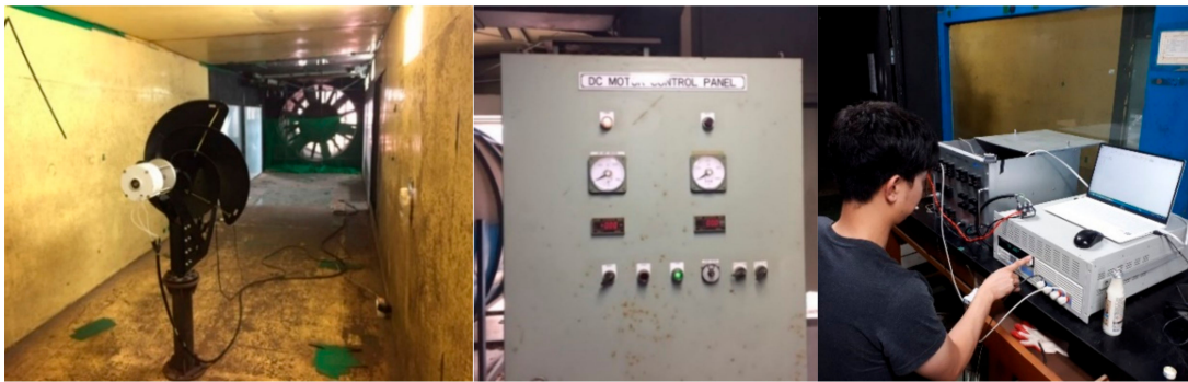
Figure 4. Installed AWM-750D and test facility.
