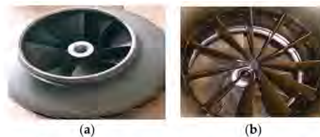
Figure 2. Compressor impeller and inlet guide vanes. (a). Impeller; (b). The IGV at the suction end of the compressor.
