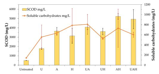
Figure 2. Comparison of different pretreatments in terms of SCOD and carbohydrates.
