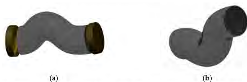
Figure 2. Physical appearance of the concerned product: (a) Product composed by a steel body tube and two polymer protections; (b) Product composed by a steel body tube.
