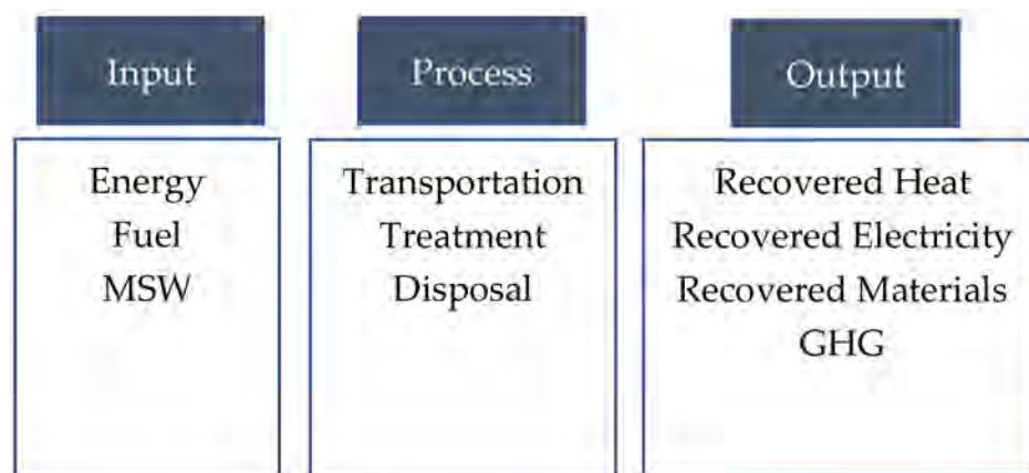
Figure A1. WtE process description. The graph is based on reference [75].
