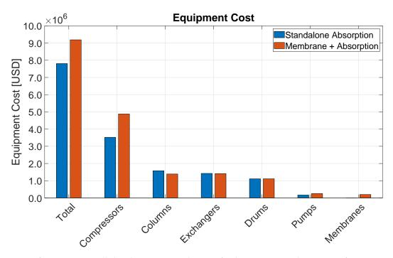
**Figure 8.** Cost of equipment installed in the CO<sub>2</sub> removal section for the two compared process configurations. Reproduced with permission from Penteado, Ph.D. Thesis, TUB, 2021 [25].
