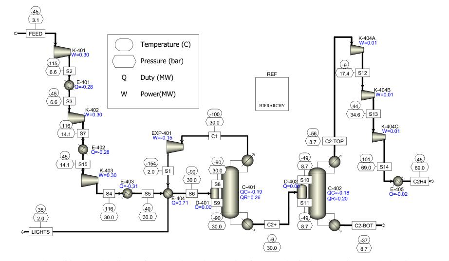
Figure 9. Process simulation of the traditional distillation configuration implemented in Aspen Plus software. Reproduced with permission from Penteado, Ph.D. Thesis, TUB, 2021 [25].
