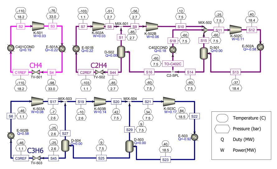
**Figure 10.** Process simulation of the external refrigeration system of the traditional distillation configuration implemented in Aspen Plus software. Reproduced with permission from Penteado, Ph.D. Thesis, TUB, 2021 [25].
