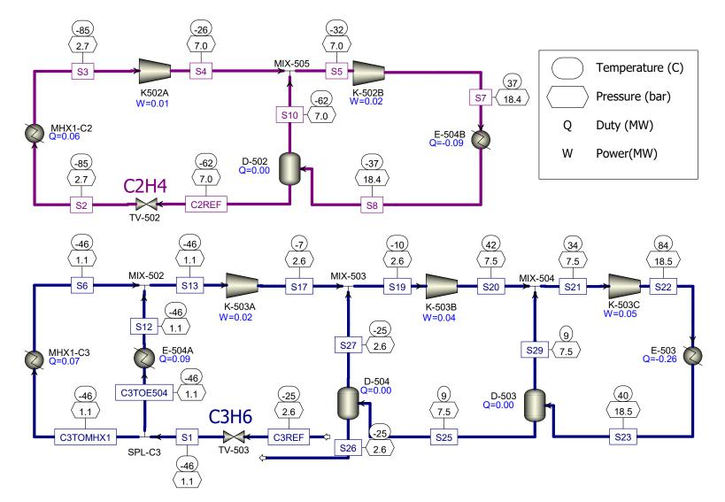
Figure 12. Process simulation of the external refrigeration system of the RSV distillation configuration implemented in Aspen Plus software. Reproduced with permission from Penteado, Ph.D. Thesis, TUB, 2021 [25].
