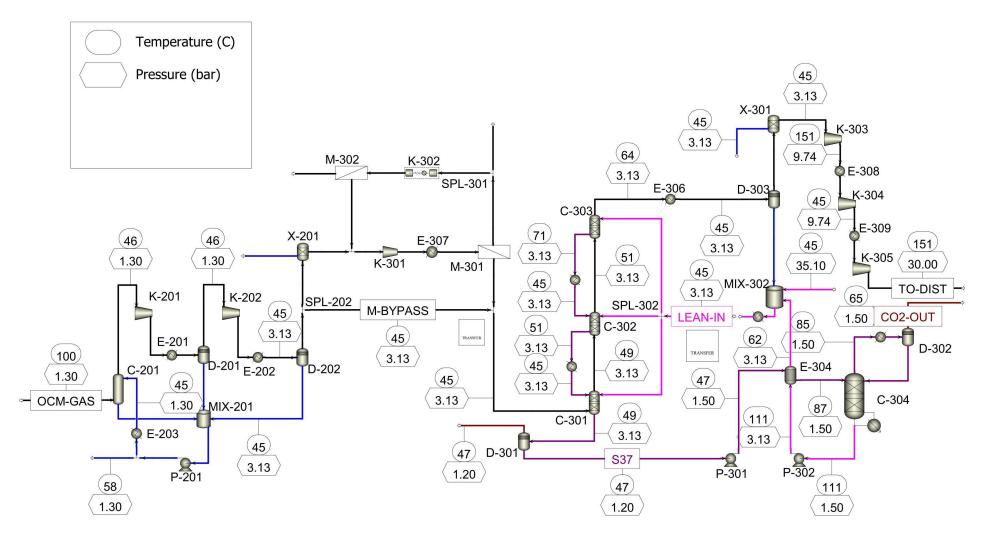
**Figure 6.** Process simulation with optimal process structure and operating conditions for the CO<sub>2</sub> removal section of the Bio-OCM plant using only absorption. Reproduced with permission from Penteado, Ph.D. Thesis, TUB, 2021 [25].
