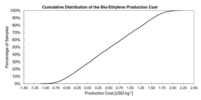
Figure 15. Cumulative distribution for the bio-ethylene production cost resulting from the Monte Carlo simulation.
