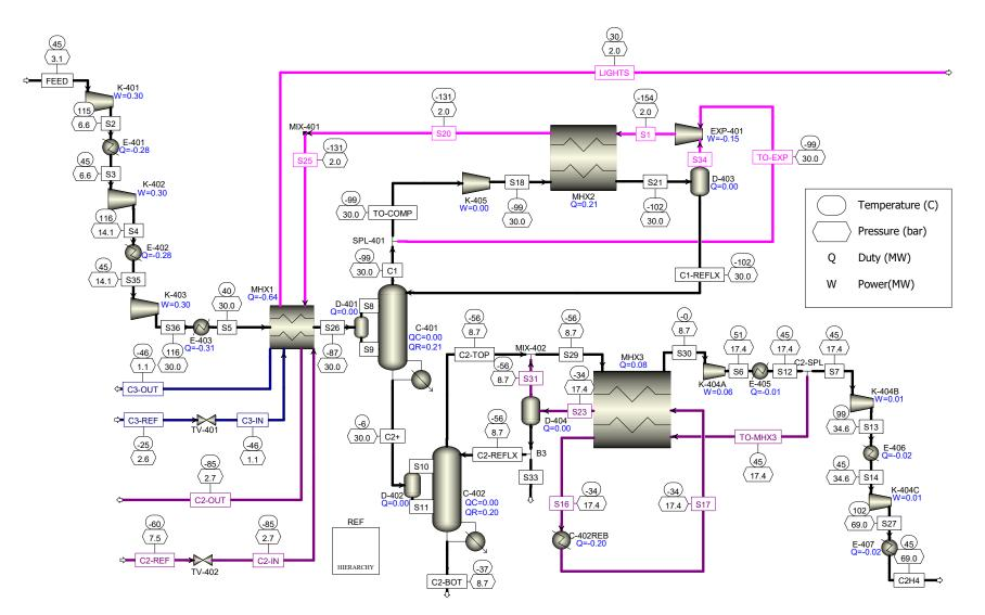
Figure 11. Process simulation of the RSV distillation configuration implemented in Aspen Plus software. Reproduced with permission from Penteado, Ph.D. Thesis, TUB, 2021 [25].
