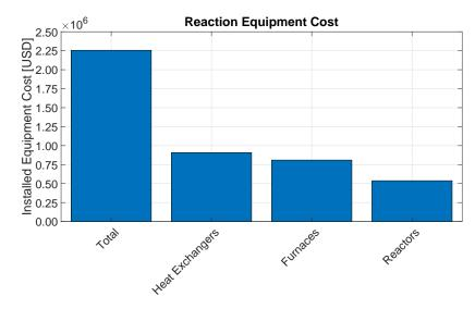
**Figure 5.** Estimated cost of equipment installed in the reaction section of the Bio-OCM plant. Reproduced with permission from Penteado, Ph.D. Thesis, TUB, 2021 [25].
