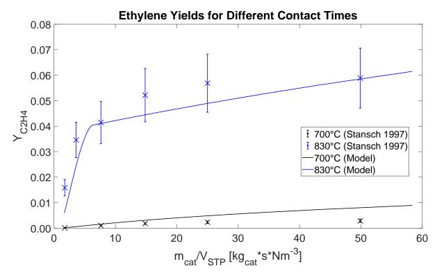
**Figure 2.** Product (C<sub>2</sub>H<sub>4</sub>) yield for different contact times obtained with an OCM-PBR operated isothermally at 700 °C and 830 °C. Reactor model predictions compared to experimental data from [7]. Reproduced with permission from Penteado, Ph.D. Thesis, TUB, 2021 [25].
