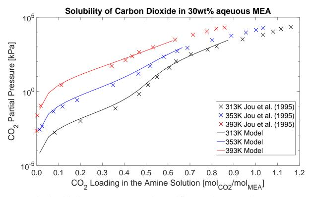
**Figure 3.** Carbon dioxide loading in 30 wt% MEA water solution at different partial pressures and temperatures. Comparison of values predicted by the developed model and experimental data from [34]. Reproduced with permission from Penteado, Ph.D. Thesis, TUB, 2021 [25].
