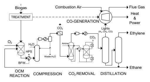
**Figure 1.** Process flow diagram of the Bio-OCM process. Dashed lines represent optional streams and units. Reproduced with permission from Penteado, Ph.D. Thesis, TUB, 2021 [25].
