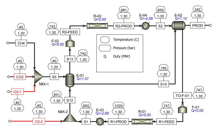
**Figure 4.** Process simulation with optimal operating conditions for the reaction section of the Bio-OCM plant carried out in Aspen Plus software. Black lines (process streams) and red lines (oxygen streams). Reproduced with permission from Penteado, Ph.D. Thesis, TUB, 2021 [25].
