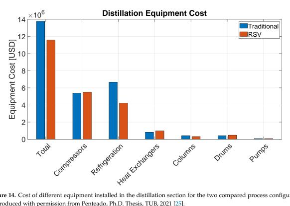
Figure 14. Cost of different equipment installed in the distillation section for the two compared process configurations. Reproduced with permission from Penteado, Ph.D. Thesis, TUB, 2021 [25].
