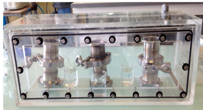
Figure 2. Picture of the airtight container for filter conditioning at controlled temperature and humidity conditions.
