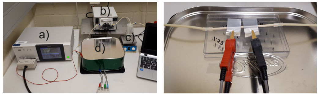
Figure 2. (left): Test setup with the (a) HIOKI IM3536 LCR meter, (b) peristaltic pump, (c) magnetic stirrer and (d) the test cell, covered in the faraday cage. (right): test cell.
