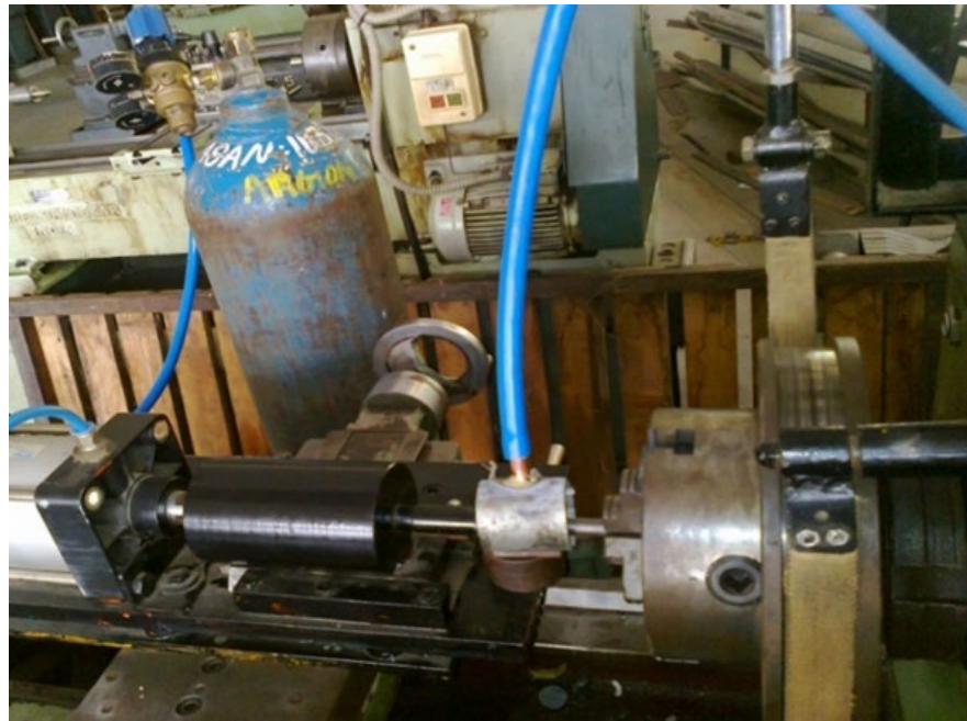
Figure 2. Experimental arrangement for friction stud welding in an inert gas atmosphere.
