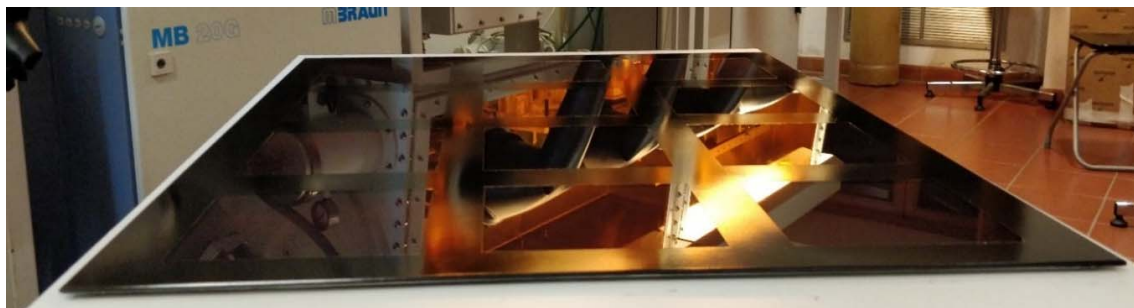
Figure 4. On the (left), backsheet insertion on the panel; on the (right), panel ready to be laminated.
