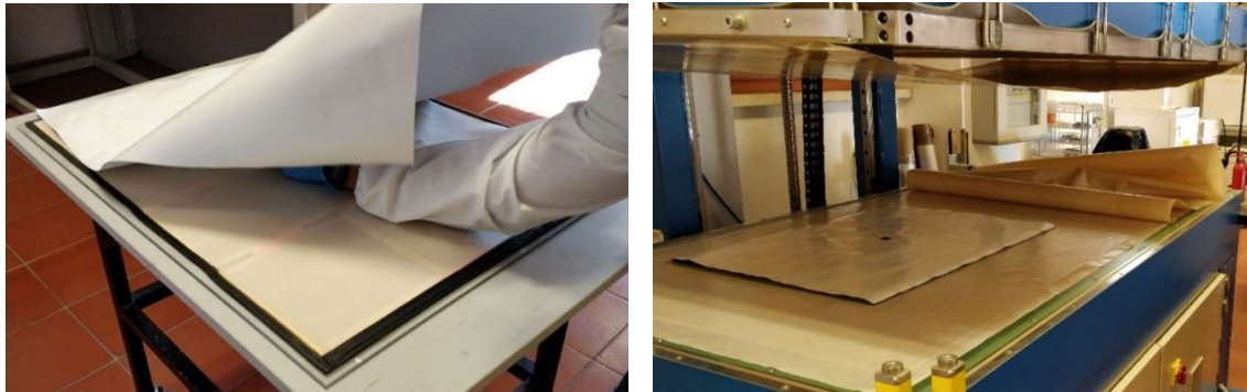
Figure 4. On the (left), backsheet insertion on the panel; on the (right), panel ready to be laminated.
