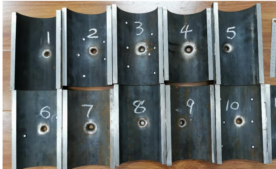
Figure 5. Internal perforation shapes in tests 1–10 after erosion.
