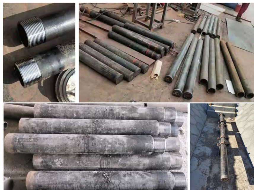
Figure 3. Photos of steel casing processing.
