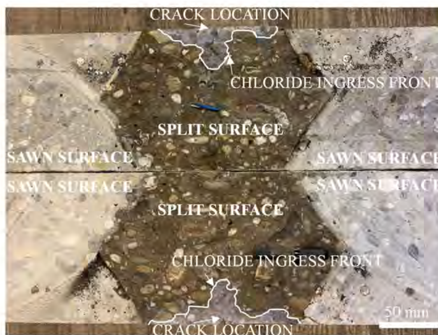
Figure 4. Visualization of the chloride ingress front on both surfaces obtained after splitting open of the beams.
