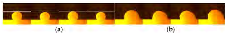
Figure 12. Behavior of the Asm-1610-60 slag droplet upon reduction (a) in the slow stage before 40 min and (b) in the rapid stage after 40 min.
