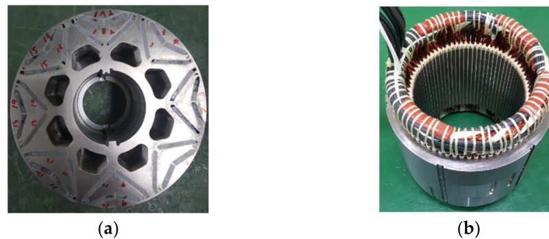
Figure 18. Topologies of the manufactured model: (a) rotor; (b) stator.
