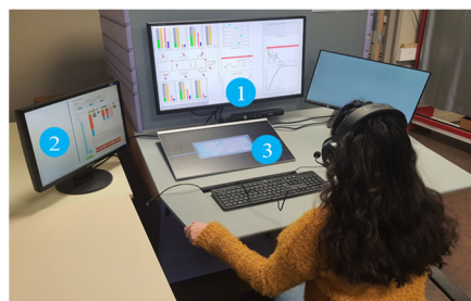
Figure 4. Production workplace (Organization 2). (1) Production control interface; (2) Planning interface; (3) Bird's eye view of the production cell.
