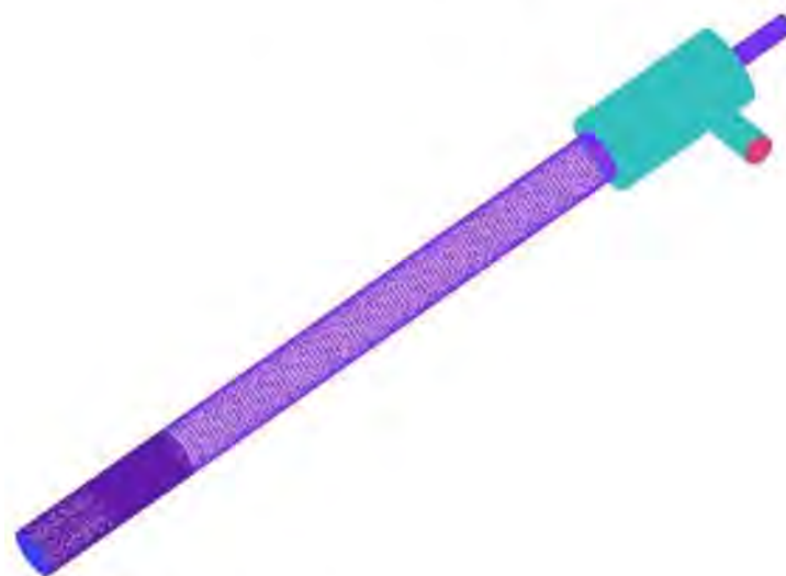
Figure 3. Mesh model of the separator.
