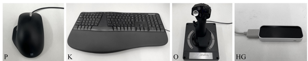
Figure 5. Input devices. (P) Pointing device. (K) Keyboard. (O) Orientation. (HG) Hand-free gesture.
