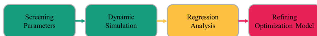
Figure 1. Tool chain to identify most influencing factors concerning the charging, storage, and discharging process.
