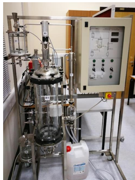
Figure 3. The pilot plant (UPB/EV-Elettronica Veneta) used in biodiesel production.
