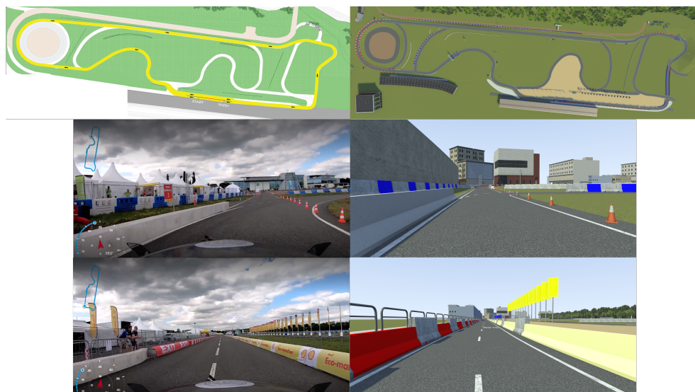
Figure 5. Numerical model of the track. Comparison between real and virtual environments.
