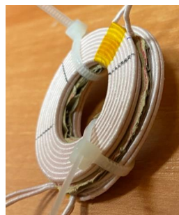
Figure 2. Air transformer under test.
