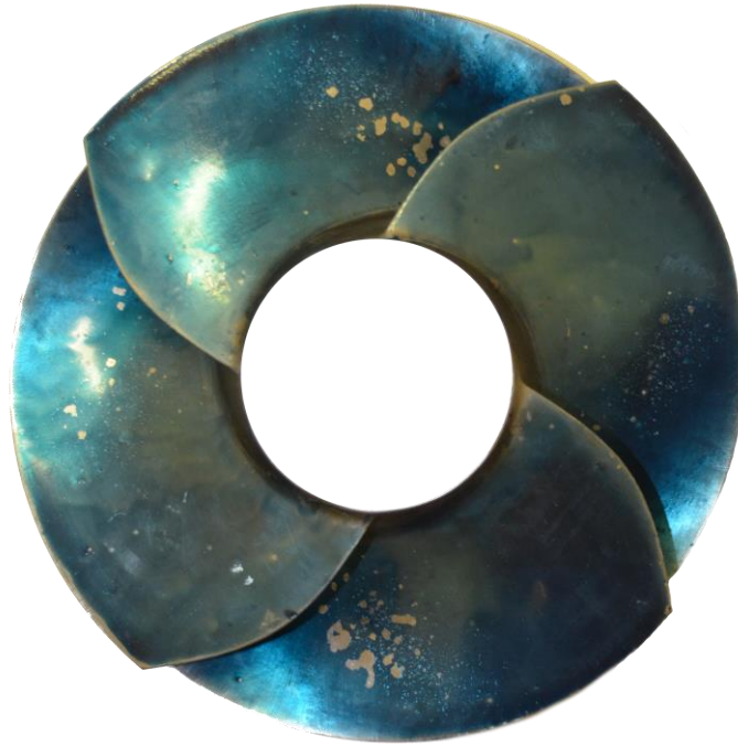
Figure 8. Cavitation erosion zones on the suction surface of rimless impeller № 2 ( Q = 0.3 \times Q_{BEP} , NPSH = 3.65 m).
