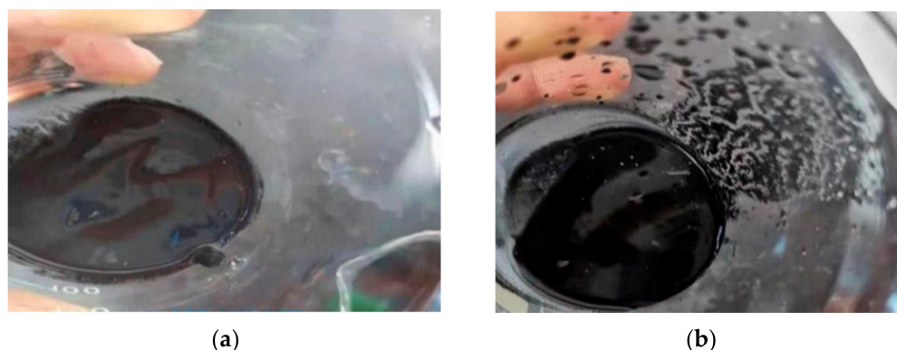
Figure 15. Appearance of sludge in the EGSB and IC reactors. (a) Sludge in the EGSB reactor. (b) Sludge in the IC reactor.
