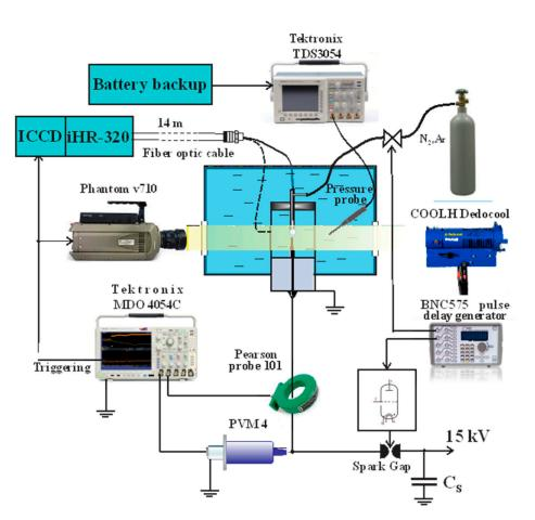
Figure 1. Experimental setup for spectroscopy investigation of spark discharge in water.
