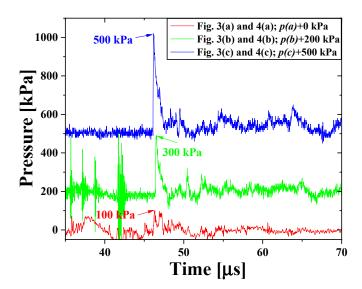
Figure 5. Pressure waveforms of a shockwave as a function of time.
