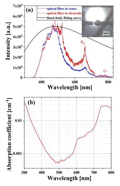
**Figure 2.** (a) Optical emission spectra of underwater spark demonstrating the effect of water on spectroscopy measurements and black-body radiation fitting curve. Inset shows the image of injected nitrogen bubble before the breakdown. (b) Measured optical absorption of used tap water.
