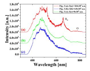
**Figure 4.** Optical emission spectra obtained from the discharge initiated in the different sizes of nitrogen bubble, using the optical fiber mounted in the cathode. The individual spectra are normalized (multiplied to have the same maximum value) and shifted vertically.
