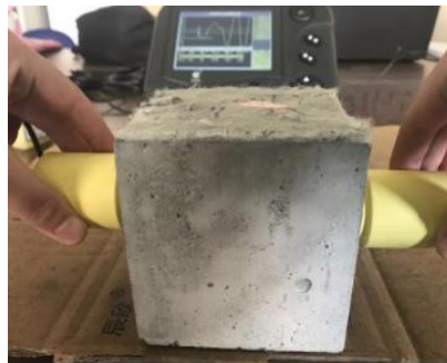
(b) Ultrasonic pulse transmission time measurement.
