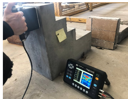
Figure 3. MIRA A1020 set-up.
