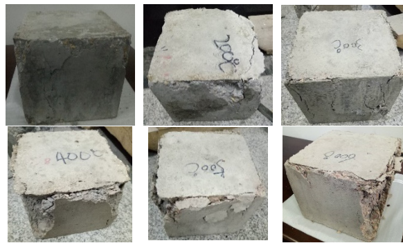
Figure 2. Typical test blocks under exposed temperatures (200 to 800 °C).
