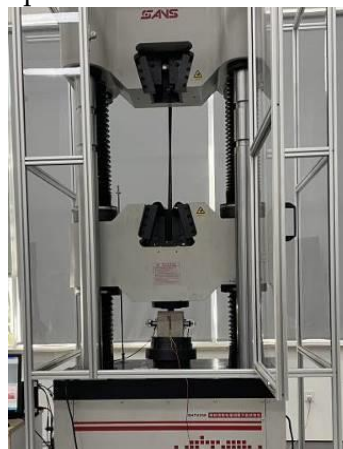
(c) Compressive testing machine.
