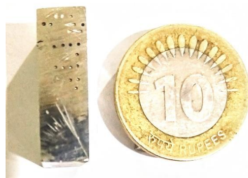
Figure 3. Fabricated microholes on the AISI 216 SS workpiece.
