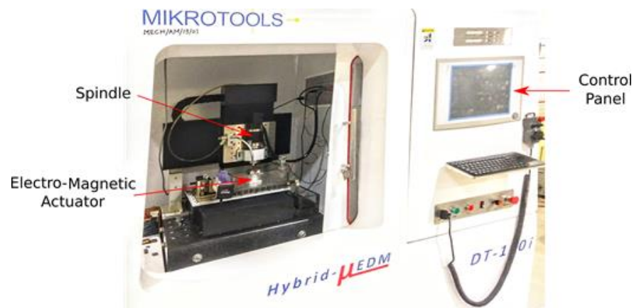
Figure 2. Micro-EDM machine used for experimentation.
