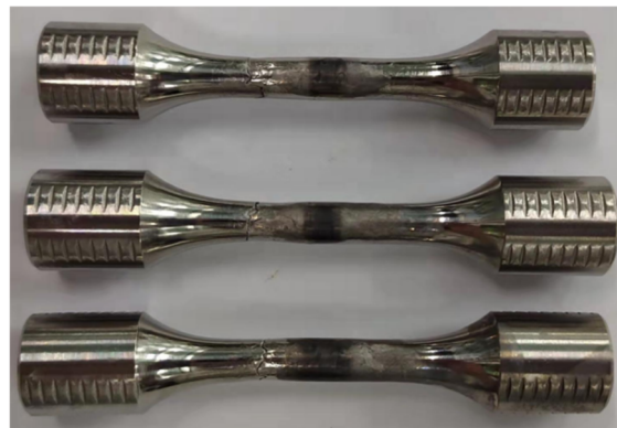
Figure 8. Diagram of tensile test samples after fracture.
