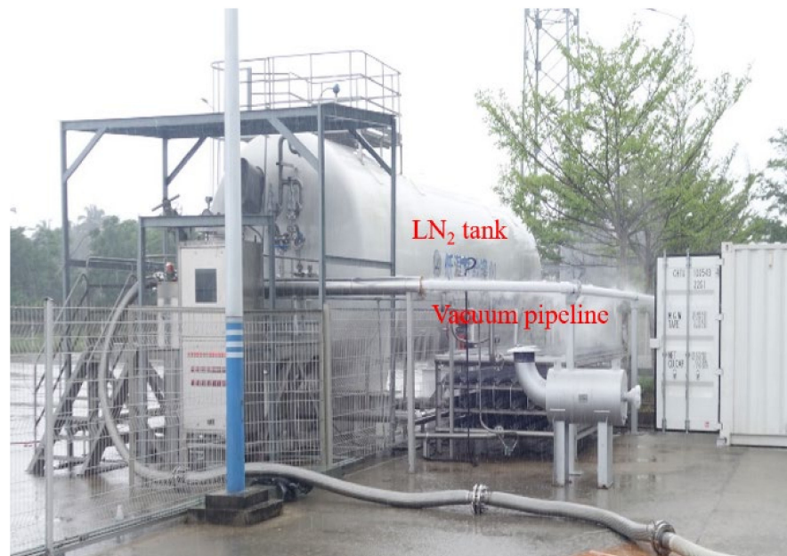
Figure 3. Image of the liquid nitrogen vacuumed subcooling test set.
