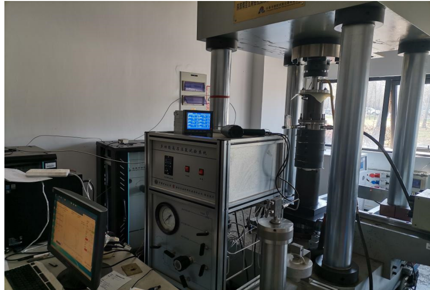
Figure 2. Coal rock mechanics-seepage test system (TAWD-2000).
