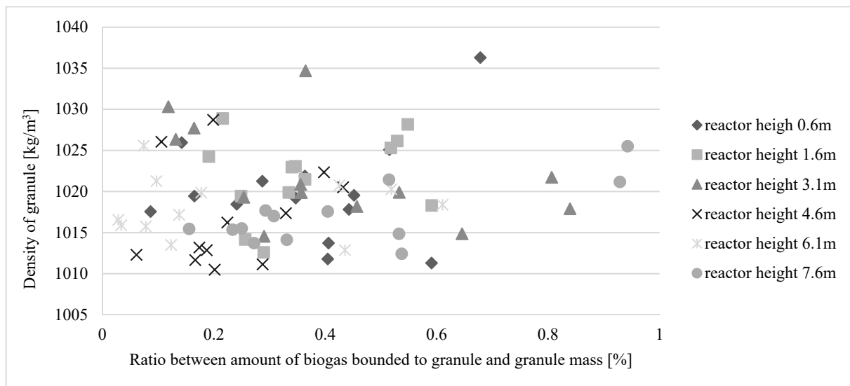
Figure 8. Ratio between the amount of biogas bound to granules and granular mass depending on the density of the granule.
