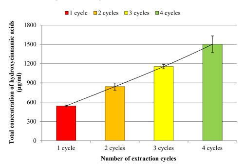
Figure 3. The effect of the number of extraction cycles on total concentration of hydroxycinnamic acids.
