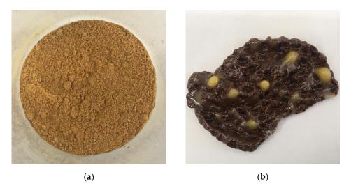
**Figure 2.** (a) Propolis before microwave-assisted extraction; (b) propolis after microwave-assisted extraction.
