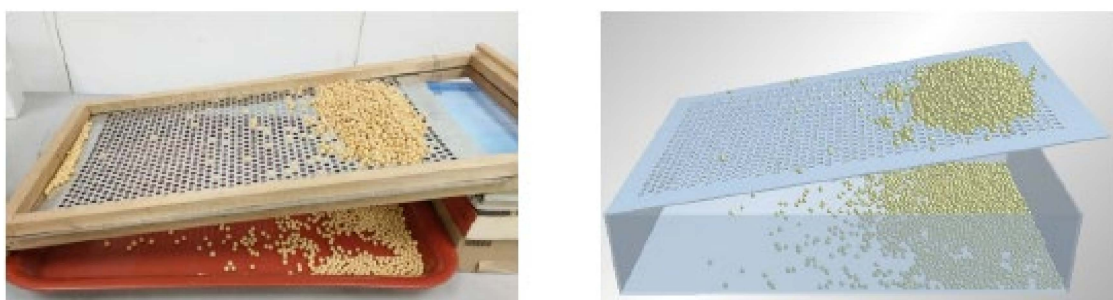
Figure 6. Test and simulation diagrams of self-flow screening.
